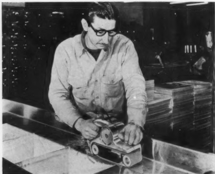
DUSTLESS SANDING: A worker smooths sheet metal surface with a Black & Decker 3-inch "dustless" belt sander. B&D claims it eliminates over 90 pct of dust and fine metal powder generated during sanding.
